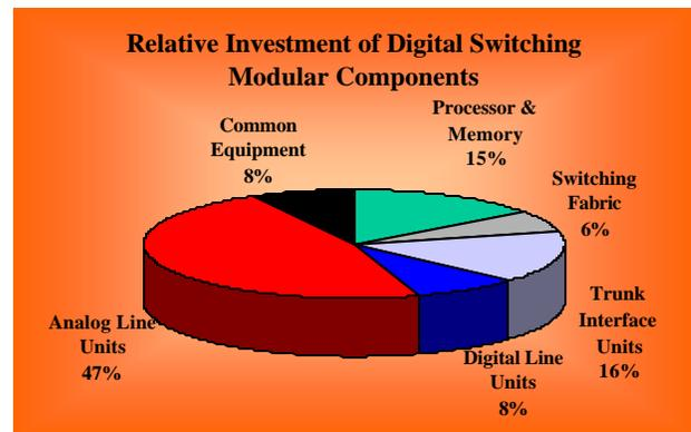
displacement of non-DLC and DLC telephone lines by IDLC technology, presented earlier. As a telephone line is upgraded to IDLC, the analog line card that connects the line to the digital switch must be replaced with integrated digital line cards (DLU).
