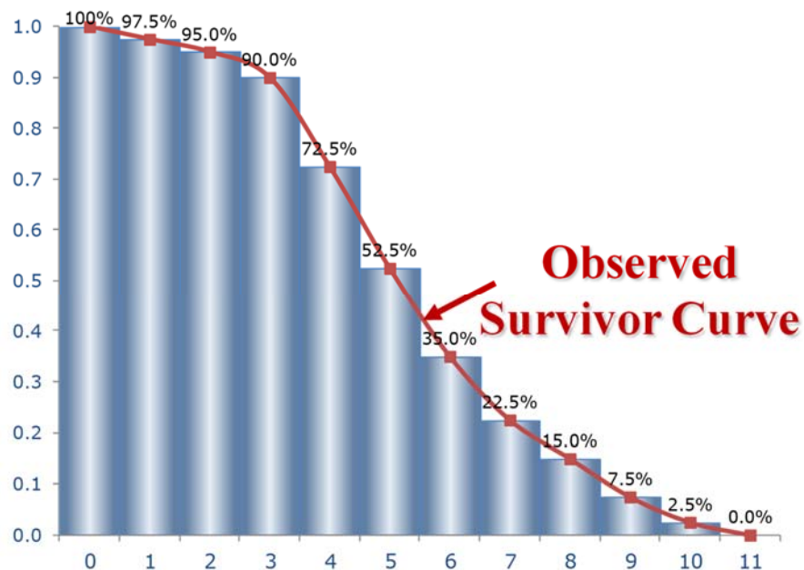
Figure 3 – Development of the Observed Survivor Curve from the Mortality Record of Experience.
